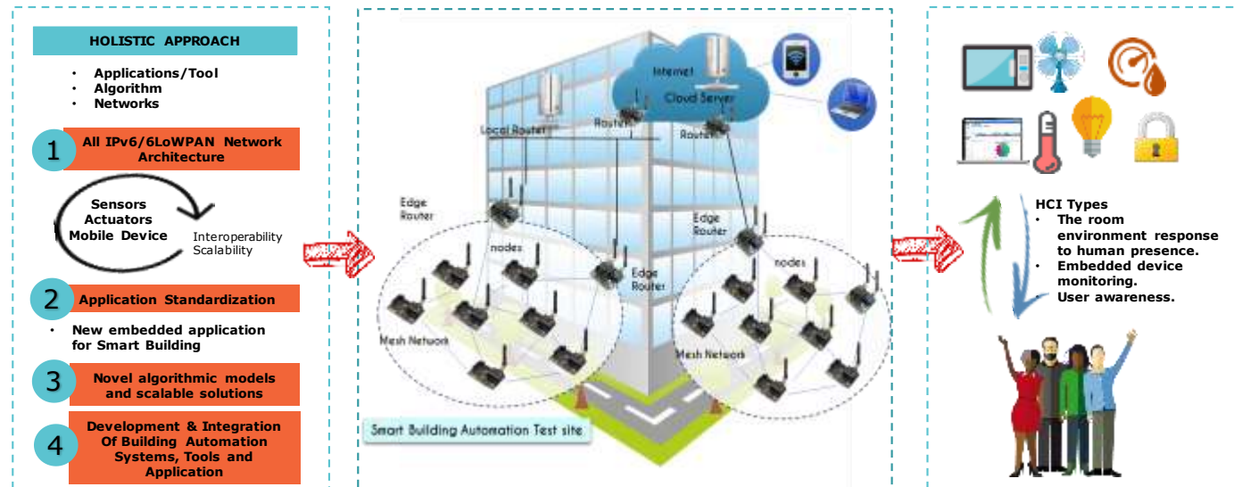
Figure 2: The SBA Platform Structure
